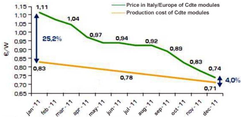
Figure 5: Evolution of the sale price and the full cost of industrial CdTe modules in 2011
