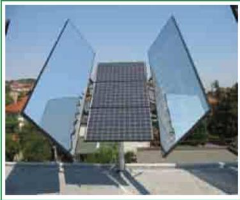
Figure 19: Low concentration PV system
